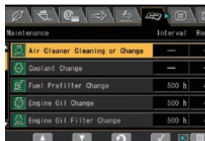
A multifunction monitor displays and controls a wealth of operational and maintenance information
