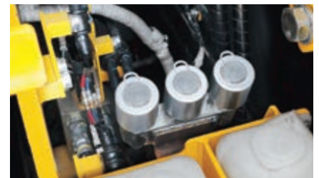
Canister-type breathers facilitate checking and cleaning
