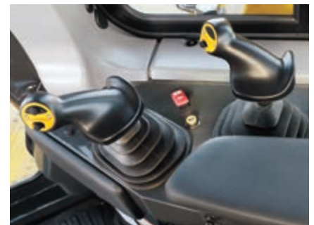
Blade control lever with auto-pitch and new ripper control lever with auto-return function
