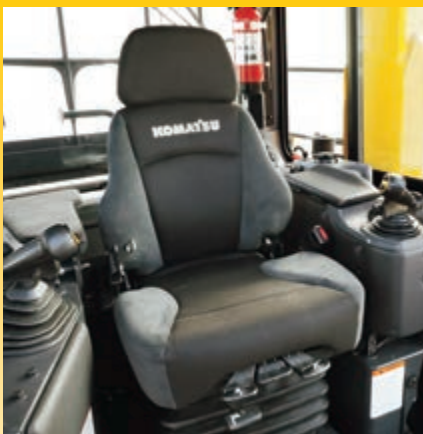
The seat is now fixed at a 12° angle to allow highest comfort for dozing and ripping.
